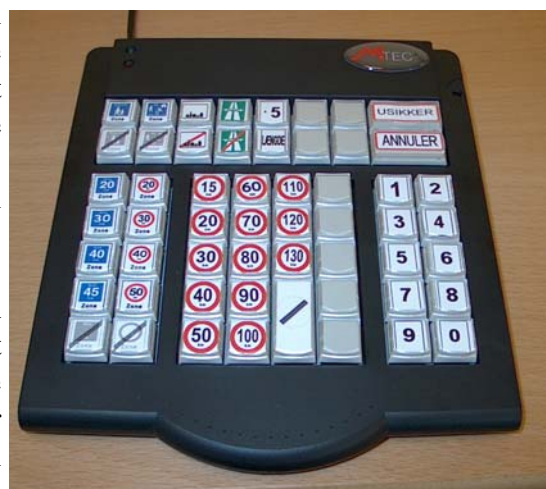
Figure 4 — Special designed keyboard for registration speed sign
