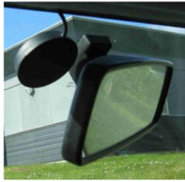
GPS Antenna placed behind the rear-view mirror
