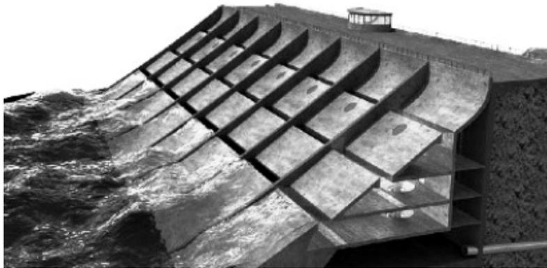
**Figure 1. Scheme of Seawave Slot-Cone Generator (SSG).**
