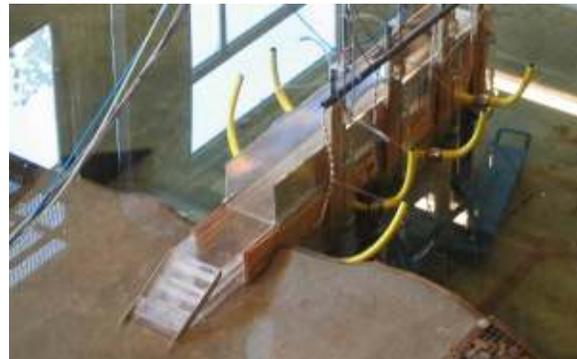
**Figure 9:** Model for 3D overtopping tests.
