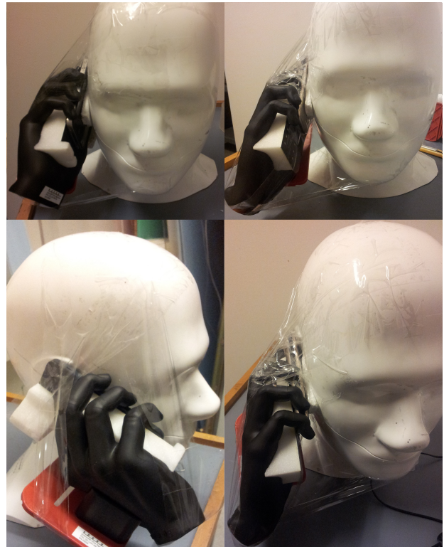
Fig. 1. The head and hands phantoms, the PDA hand on the left and the monoblock hand on the right.
