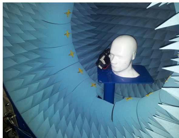
Fig. 2. Illustration of the SAM and hand phantom placement in the Starlab chamber for obtaining the TRP and TIS results.
