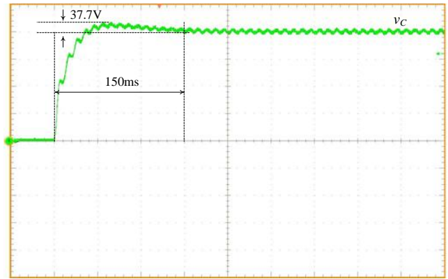
(d) Startup transient under the full load condition with 660 \mu F E-Caps ( v_C : 100V/div, Timebase: 50ms/div).
