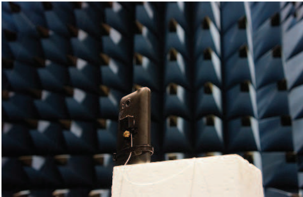
Fig. 4. Measurement set-up with optic fibers.
