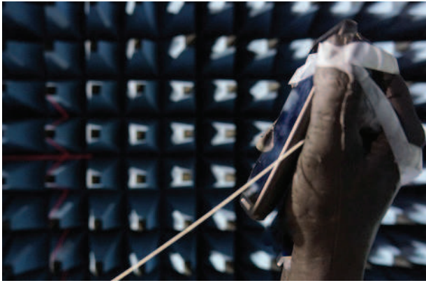
Fig. 5. Measurement set-up with optic fibers and a user's hand model.
