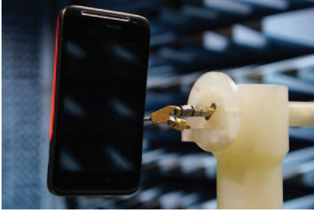
Fig. 3. Measurement set-up with a coaxial cable.
