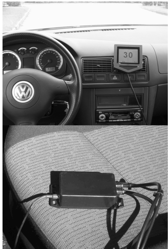
Fig. 3. The ISA equipment consisting of the display in the air nozzle (above) and the On Board Unit (below).
