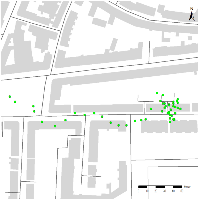
Figure 1 A visualisation of a sample from the output generated by a single GPS receiver. The sample contains 61 points which is equivalent to a time span of approximately 8 minutes and 8 seconds.
