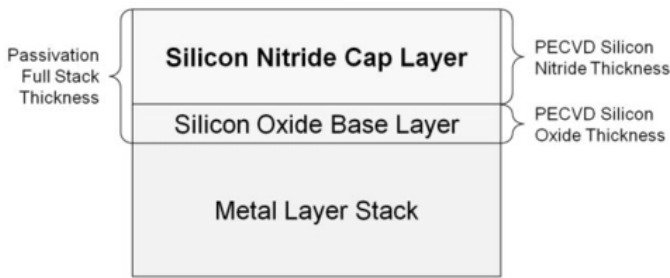
Fig. 1. Metal Passivation Layer Structure: Silicon Nitride cap layer and Silicon Oxide base layer, deposited in a PECVD process sequence for passivation of the underlying metal layer stack.
