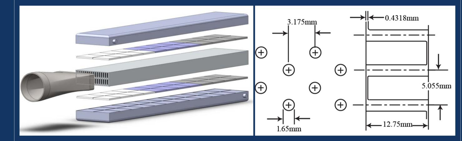
The idea here is to recover the exhaust gas heat for electricity: a TEG subsystem needs to be designed, modeled and optimized:
