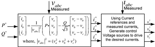
Fig. 4 Determination Voltage Source model for WTG with FSC
