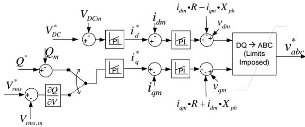
Fig. 3 Block Diagram of Onshore VSC Controller
