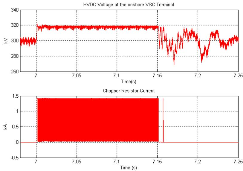
Fig. 10 Low Voltage Fault Ride through using chopper resistors.
