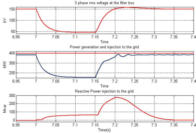
Fig. 9 Response during the low voltage fault at the PCC
