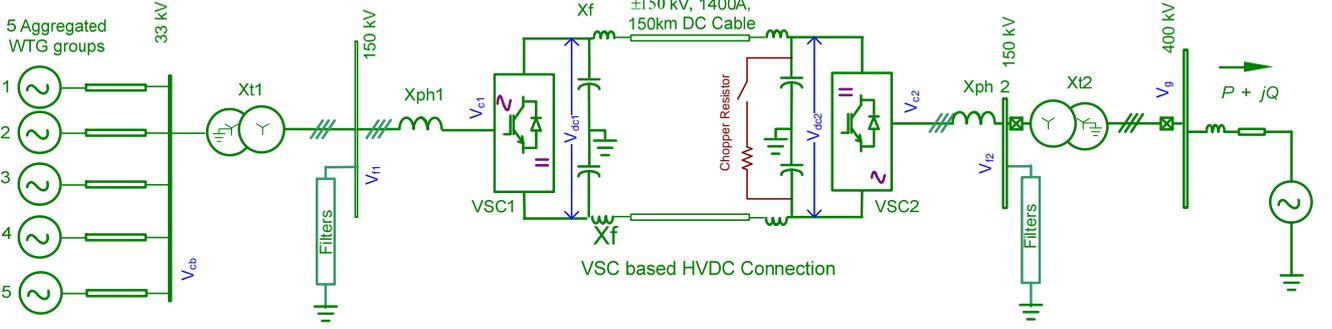
Fig. 1 WPP with VSC-HVDC connection to the grid
