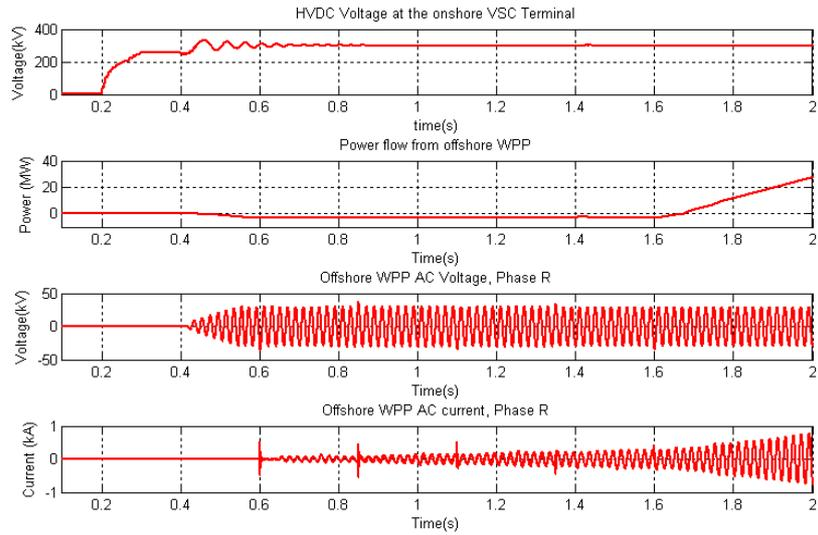
Fig. 6 Charging VSC-HVDC and energizing the offshore grid
