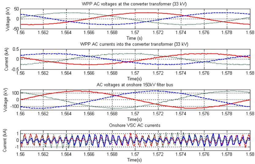
Fig. 7 Steady state operation at no load
