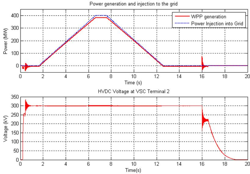
Fig. 5 Power generation and transmission and HVDC Voltage curves for a whole range of operation from start-up to shut-down.
