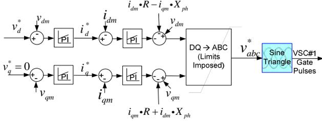
Fig. 2 Block Diagram of Offshore VSC Controller
