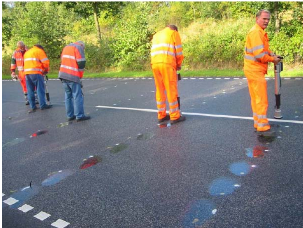
FIGURE 1 Measurements with SOBO20 portable salinity testers, at each subsection five cross-sections 2 meters apart were measured by every 0.5 meter.
