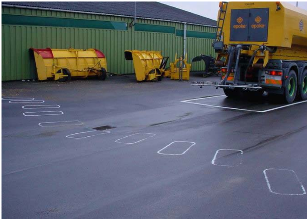
1 2 FIGURE 5 FAV’s site for verification of nozzle-spreaders. Tubs are placed on the 10 3 marked fields, one for each of the nozzles. The amount and distribution of brine spread 4 within a period of time is established simply by weighing or by measuring the height of the 5 liquid in each tub. 6
