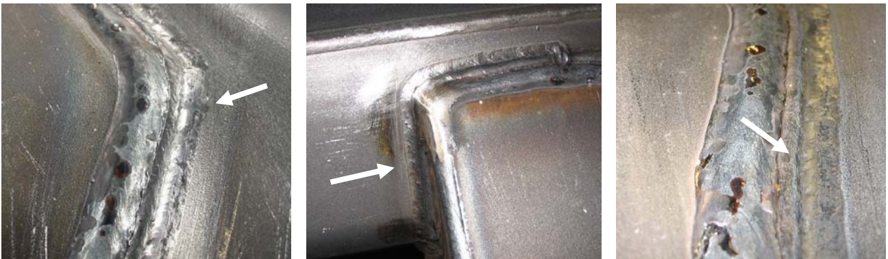
Fig. 18: Examples of final production quality TIG dressing, free from undercutting and significant imperfections.
