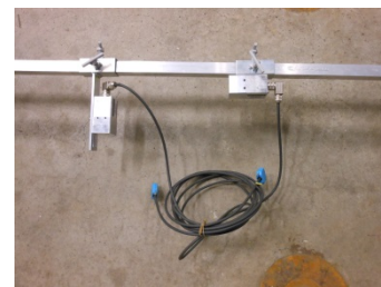
Figure 6. Displacement transducers WS10-1 and WS10-2 connected to the horizontal bar.
