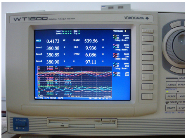
Fig. 13. Measured peak efficiency of Topology B when V_{in} = 417 V.
