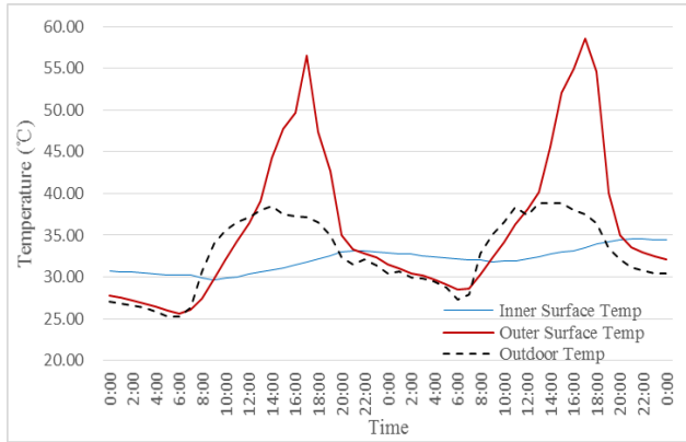
Fig. 3 Surface temperatures and outdoor temperatures measured during case 1 without night ventilation
