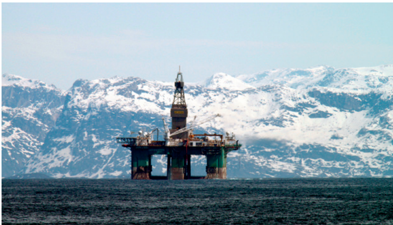
The exploratory drilling rig Leiv Eiriksson off the coast of Greenland in the Davis Strait
