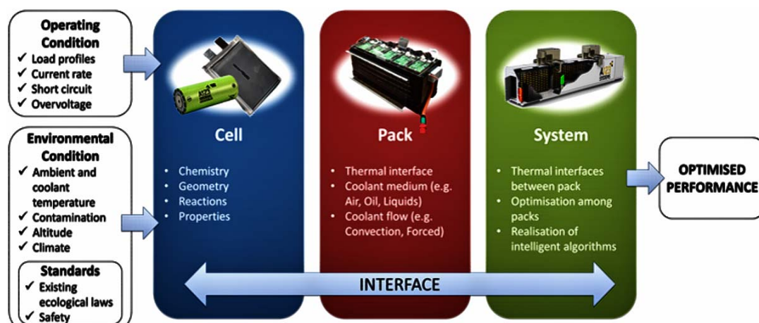
Figure 1. Battery thermal management system (BTMS).
