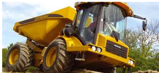
Figure 1. Hydrema 912DS Articulated Dump Truck.
