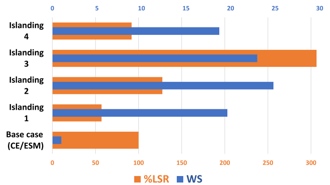
FIGURE 5. Comparison of DCOPF formulation based base case (CE/ESM) and DCOPF formulation based IIS for IEEE 39-bus system.
