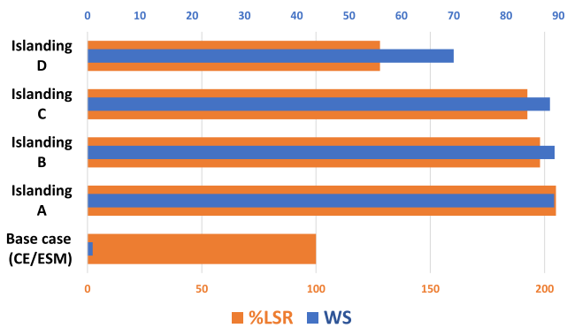
FIGURE 8. Comparison of ACOPF formulation based base case (CE/ESM) and ACOPF formulation based IIS for IEEE 118-bus system.
