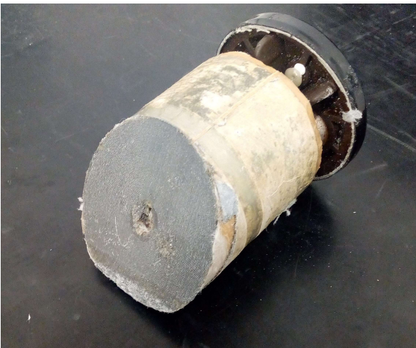
Fig. 8: Capacitor cut in half for measuring purposes.
