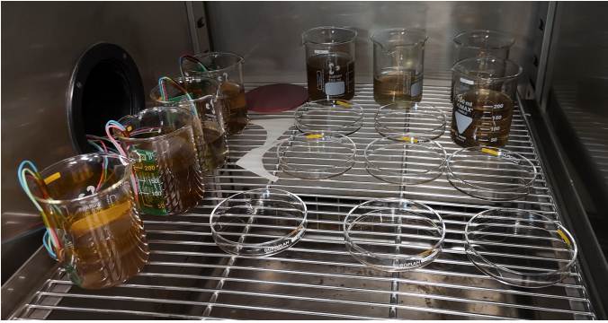
Figure 2. Climatic chamber contains the test specimens.
