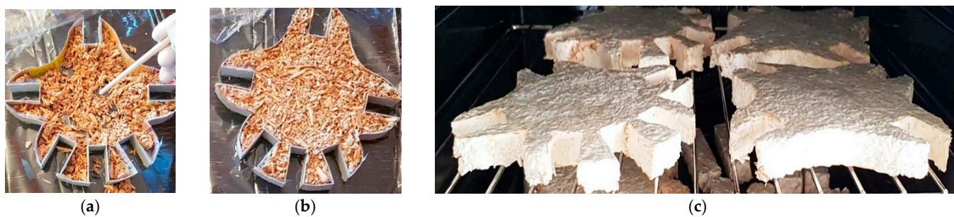
Figure 15. Production process: (a) Prefabricated molds filled with the growing material, (b) Incremental compacting for a higher density, (c) Grown samples ready to be dried in an oven.
