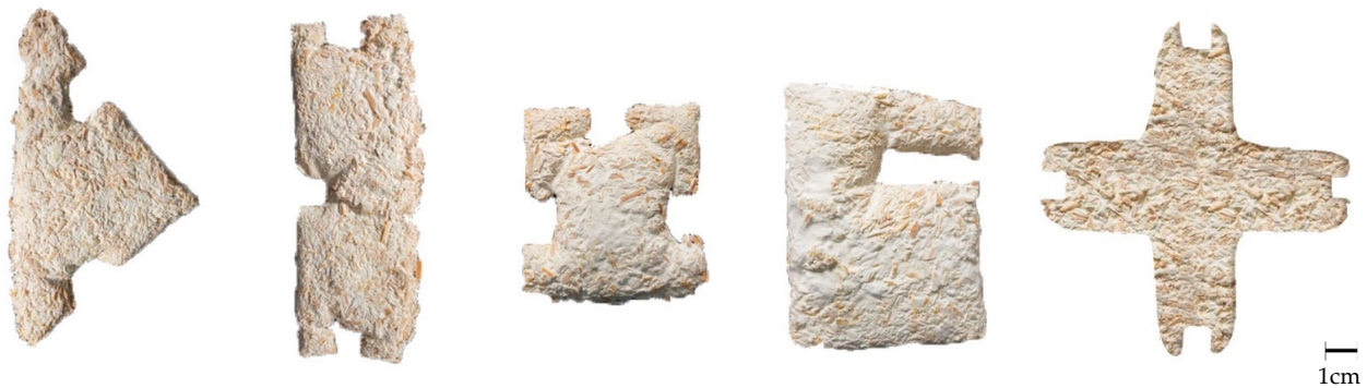
Figure 3. First experiment: modules of different shapes with embedded finger joints.
