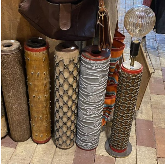
Figure 3. Antique wallpaper printing rollers. The one to the right is upcycled into a lamp. Photo from a private retro shop.
