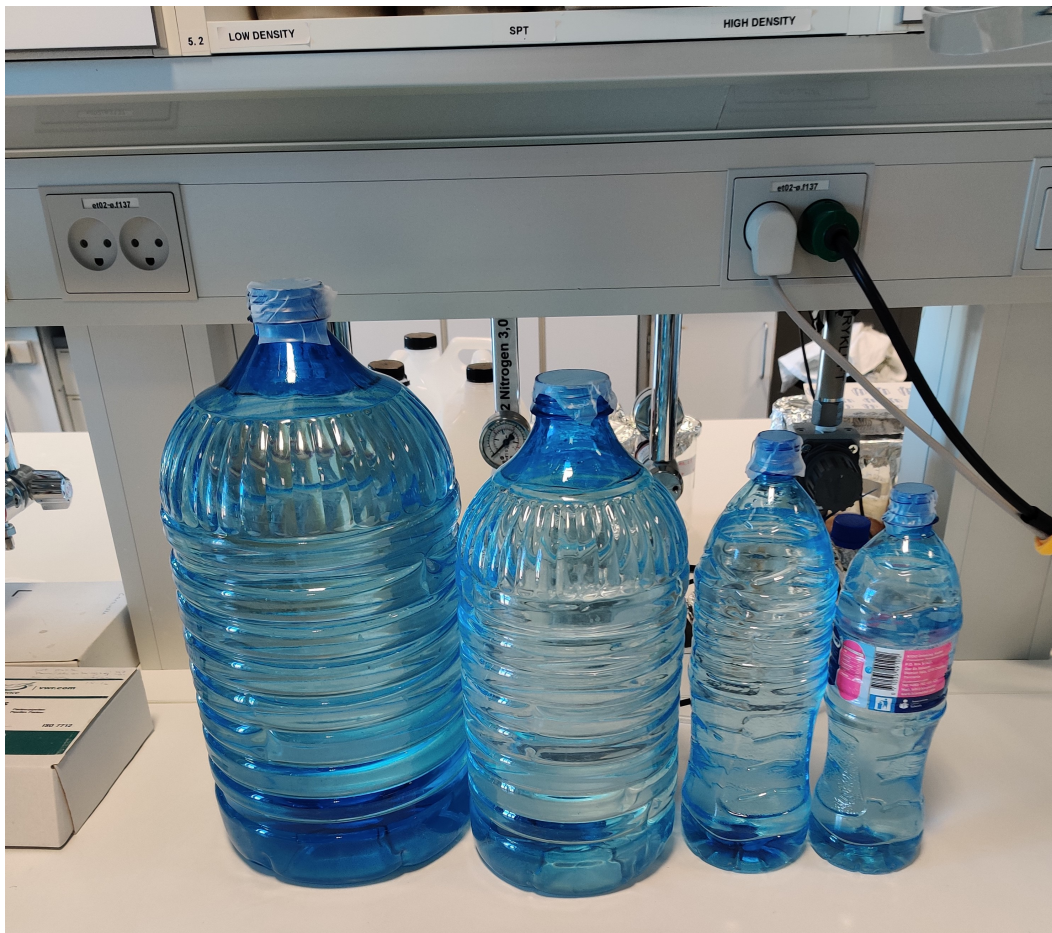
Figure 6.1. Bottle sizes used for testing from left to right; 10000mL, 5000mL, 1500mL and 1000mL.
