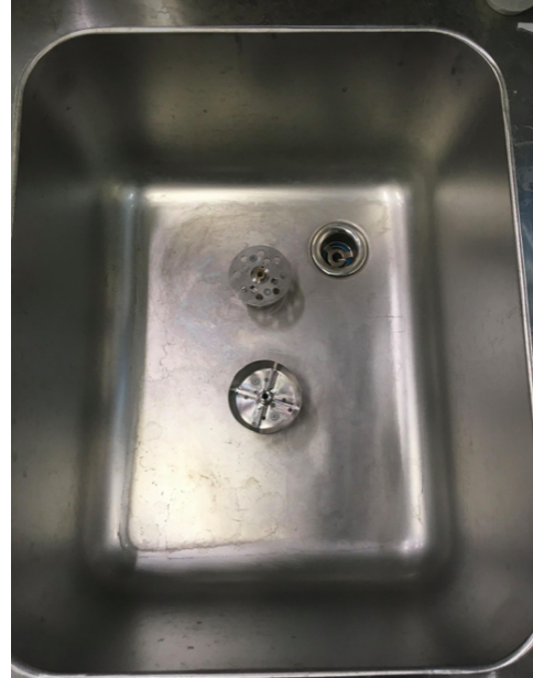
Figure 2.2. The sink with two nozzles used for cleaning the cap and the bottle respectively.
