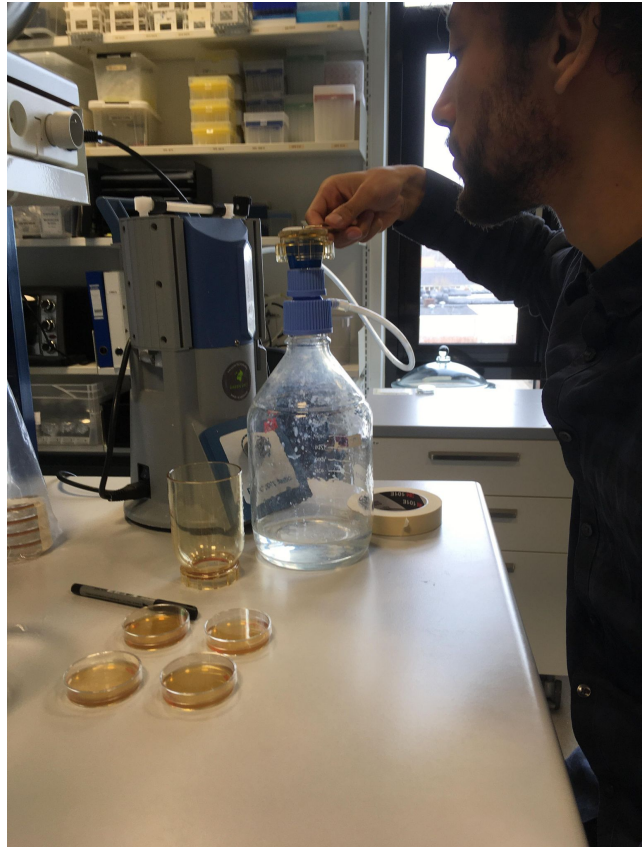
Figure 7.3. Set up of the membrane filtration apparatus, as the filter is placed.
