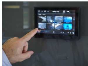
Figure 3: Smart screens panels providing access to connected devices (H6).
