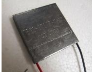
Fig. 2. BiTe based TEG used in experiments [26].
