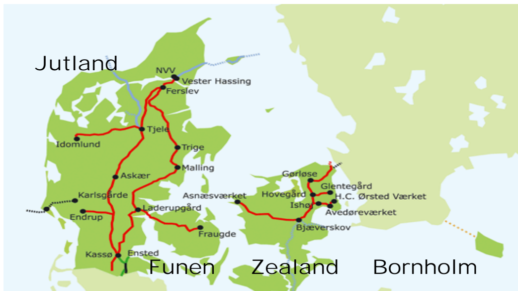
Figure 2.1 Map of Denmark with electrical power system of Energinet.dk shown. From the left, the Jutland peninsula and interconnected island of Funen (the Western part) and the other two islands are Zealand and Bornholm [www.energinet.dk]. Red 400 kV lines, blue – dc lines, orange, dotted – 60 kV cable.
