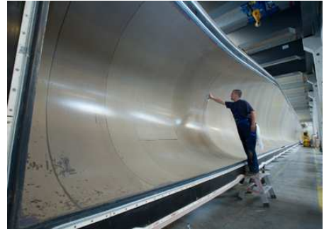
(b) Upraised part of a mold used for placing the reinforcement materials
