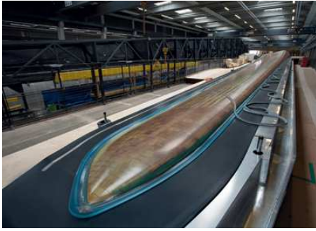
(a) A cured wind turbine blade manufactured using the VARTM process
