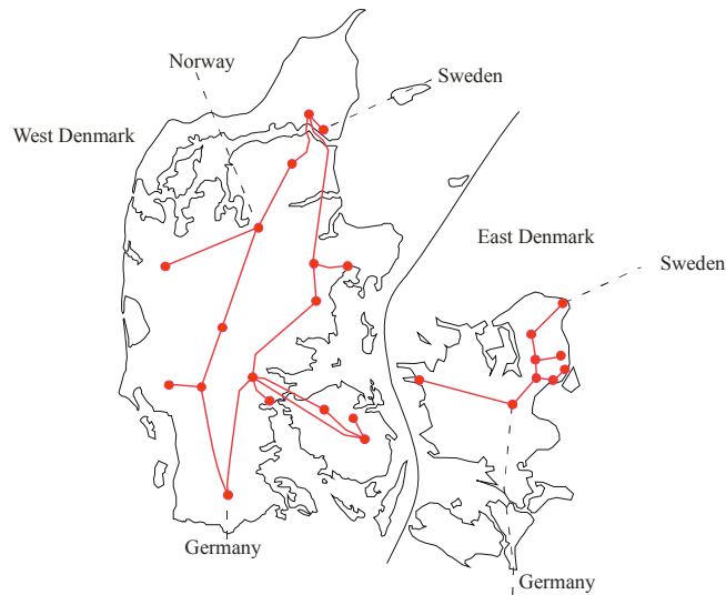
Fig. 2, The 400 kV transmission grid in Denmark and connections abroad. The two systems will connect via a DC line in the future.
