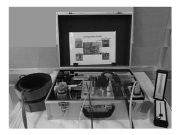
Figure 6. The computer-controlled cuff algometry.
