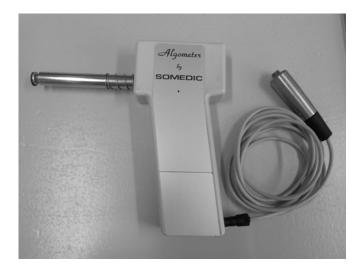
Figure 4. Hand-held (manually applied) pressure algometer.
