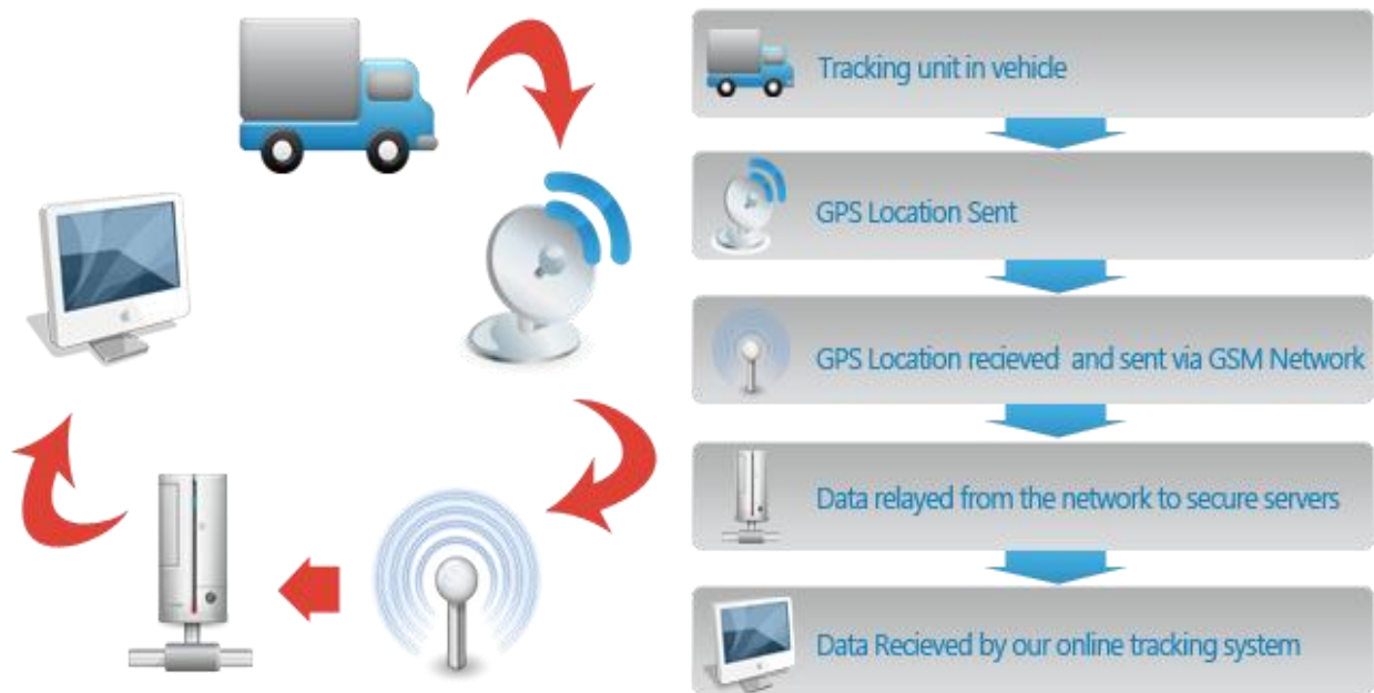
Figure 2.4: Typical Vehicle Tracking System & Tracking Process
