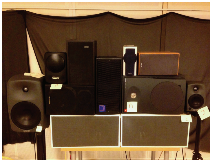
Fig. I: The “baffle” setup of loudspeakers for Test 2. The white-framed loudspeaker (lower left) was kept for symmetry, but only the right was included in the test. The large Genelec (leftmost) was placed on top of the white left loudspeaker in Test 1. The position of the two other anchor loudspeakers were fixed between Test 1 and Test 2.
