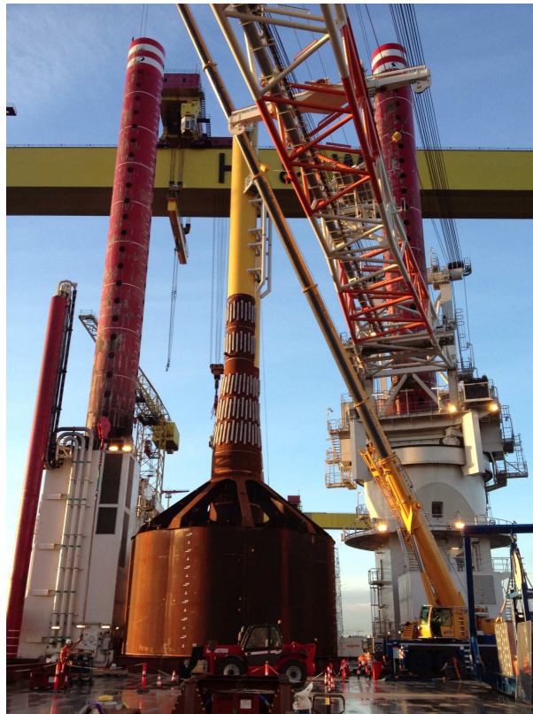
Figure 6: Real-scale monopod bucket foundation on the deck of a jackup vessel
