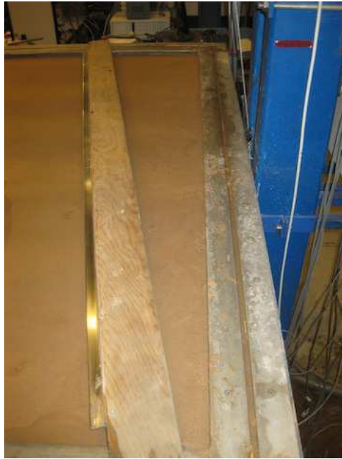
Figure 10: Lath used to smooth the soil surface
