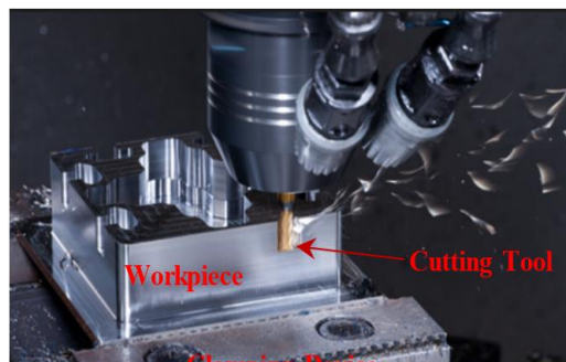
Figure 2-8: Typical machining operation performed by a CNC Milling machine.
