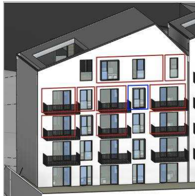
Fig. 1 Section of a multi-story residential building with rectangles indicating the possible “critical” rooms caused by different room geometries, ventilation rates, windows, and overhang. The room enclosed by a blue rectangle is used for the case study below (Illustration: AART architects).
