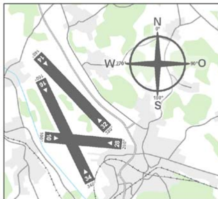
Figure 34: Runways system at Zurich Airport, with three runways, where two are intercepting which limits the capacity (Flughafen Zürich AG, 2012a)
