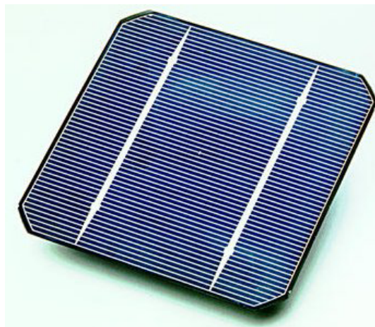
Figure 2.1. A modern mono-crystalline silicon PV cell, with a multiple of thin fingers for collecting the free electrons, and two thick bus bars for interconnection.
