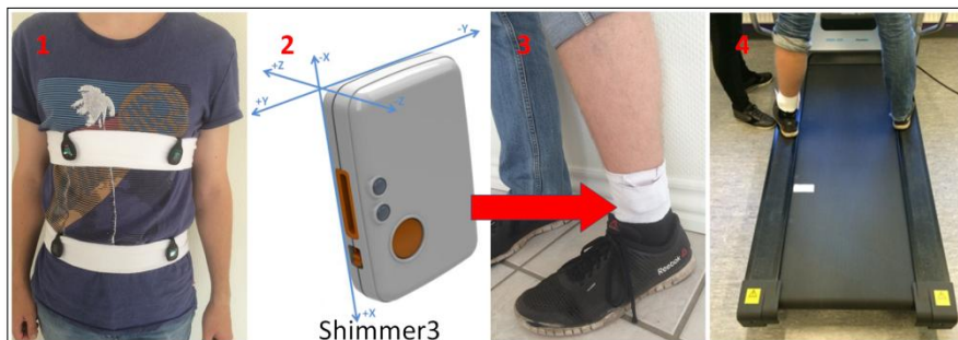
Picture 1: Placement of the four Zips. Picture 2: Shimmer3 with gyroscope range displayed in x, y and z directions (86). Picture 3: The Shimmer was placed in an elastic band on the ankle with the orientation of the gyro Z-axis perpendicular to the sagittal plane on the participant's left ankle. Picture 4: Placement of the Shimmer during treadmill walking.
