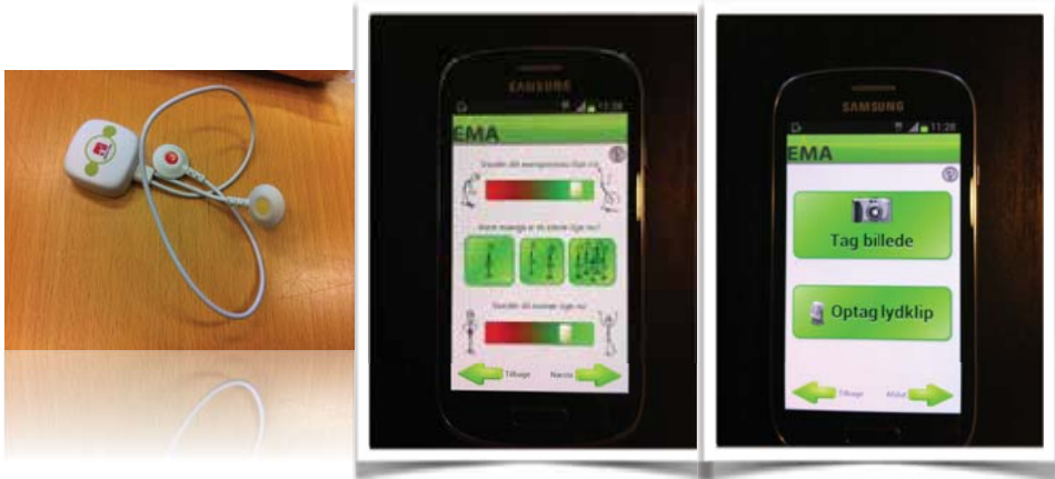
Figure 8-1: In the picture on the left, the heart rate variability monitor used for the test is depicted. The picture in the middle shows the data-logging system downloaded onto a mobile phone and the screen where the participants were able to log energy levels, number of people present in the room, and mood at the moment of logging. The picture on the right shows options of taking a picture and recording a short audio file.
