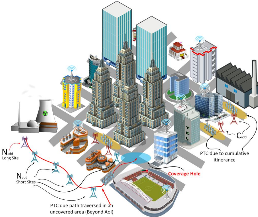
Figure 3-5-9: An AoI that is subjected to a complex network environment where multiple iterations may lead to the cumulative PTC-generating need of additional coverage and/or capacity sites
