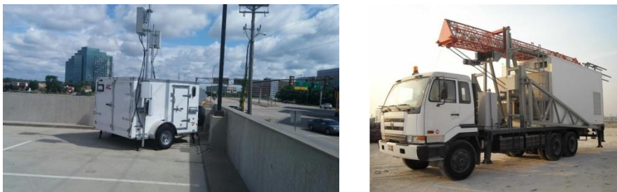
Figure 6-2-5: Cell on wheels [Source: (a) Left: General Dynamics Mission Systems, weblink: https://gdmissionsystems.com/lte/cell-on-wheels/ ; (b)Right: Advanced Communications and Electronics Systems Co. Ltd., weblink: http://www.aces-co.com/civil_cellonwheels_rd.html ]
