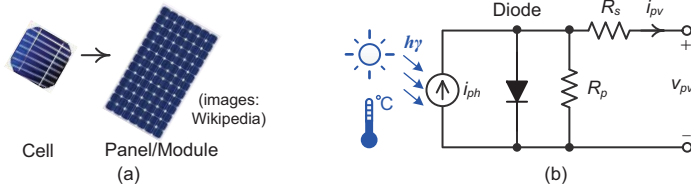
Figure 2.1: A PV module: (a) from PV cells to module and (b) PV cell model.
