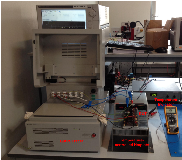
Figure 5.13: Testing setup for IGBT saturation current at different temperatures.
