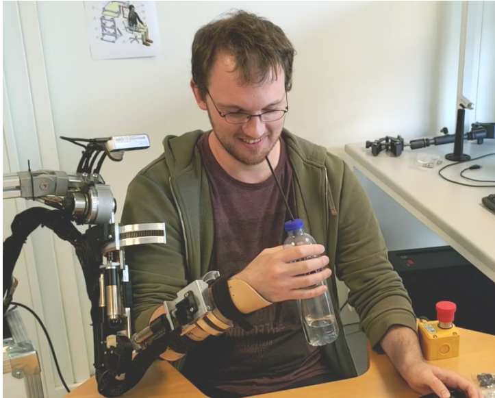
Fig. 1.1: The author drinking from a straw with the aid of an upper limb exoskeleton and glasses. Both are examples of an assistive technology but at different stages of maturity. Glasses have existed for centuries whereas exoskeletons have just recently become a possibility for assistive purposes.
