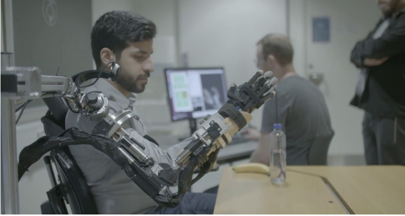
Fig. B.2: The EXOTIC exoskeleton system. An individual commands the EXOTIC exoskeleton using a tongue interface shared with computer vision based semi-automation. The individual shown in the image has given a written consent to the use of the image.
