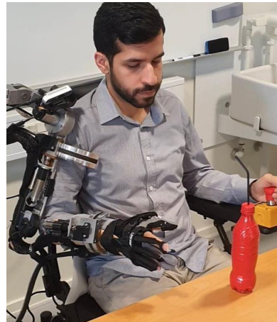
(b) A person wearing the exoskeleton and the Carbonhand. Figure adapted from [4], paper D.
