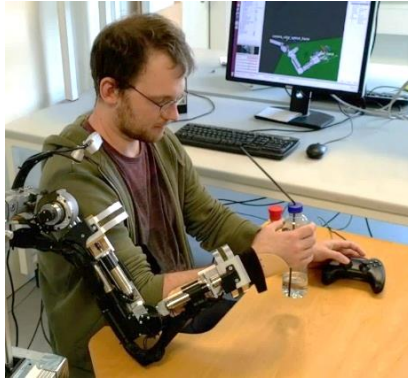
Fig. A.1: Image of the proposed exoskeleton here shown to successfully move the users hand to grasp a bottle and consecutively move it to the users mouth to sip from the straw.
