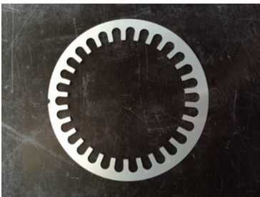
Figure A-5 Stator steel lamination
