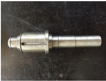
Figure A-3 Inner rotor shaft
