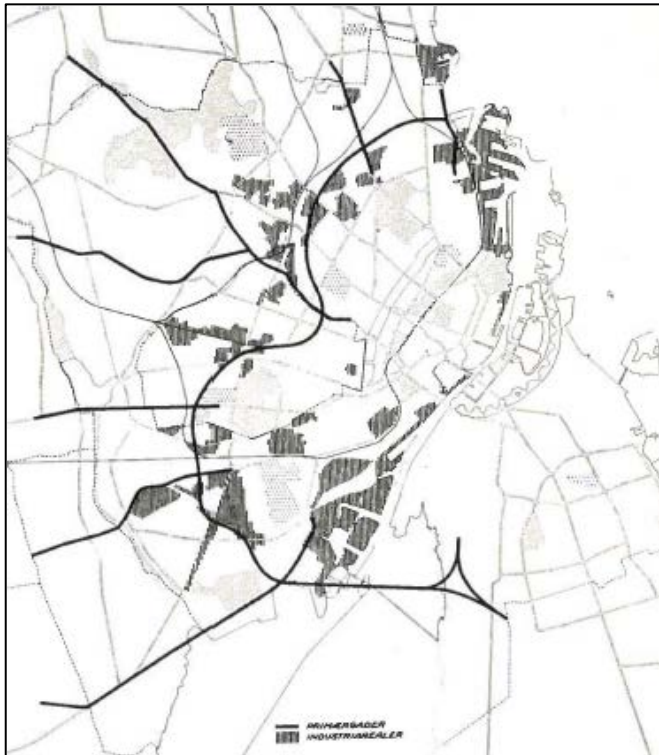
Figure 9.6: The proposed Goods-ring, running in the trace of a former goods railway (Stadsingeniørens Direktorat 1955c, p. 10)
