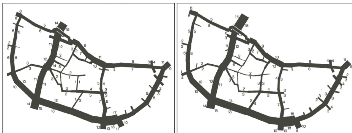
Figure 8.1: Traffic calculations for the inner city road system, both with (to the left) and without (to the right) the Dag Hammarskjöld Street breakthrough, 1990 (Nyvig A/S 1973e)
