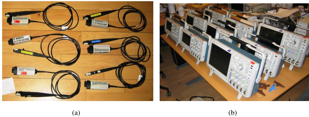
Figure 10.3: (a) Tektronix TCP0030 current probes and (b) Tektronix DPO2014 oscilloscopes.
