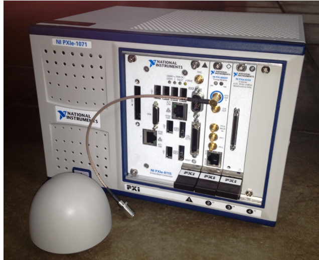
Figure 12.2: National Instrument equipment used to build fault locator unit.
