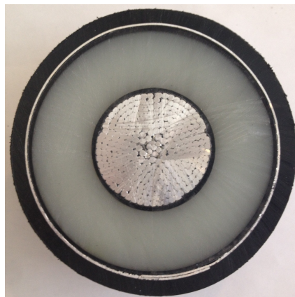
Figure 5.3: Physical layout of the 2000 mm 2 aluminium single core 245 kV cable.
