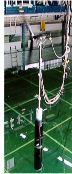
Fig. 3.15: OC3-Hywind spar buoy during testing at MARIN [Robertson et al., 2013]
