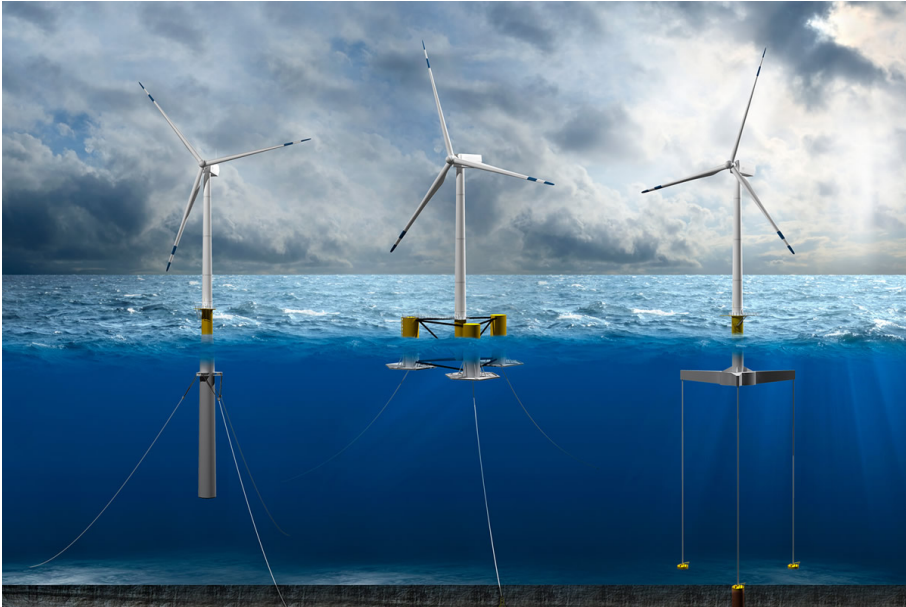
Fig. 2.2: The three archetypes of floating foundations adopted by the wind energy industry. From left: Spar buoy, Semi-Sub, TLP [DNV GL, 2016]
