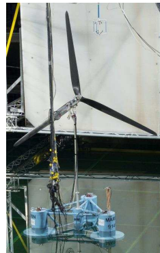
Fig. 1. DeepCwind semisubmersible system as tested in MARIN's ocean basin. Photo by Andy Goupee, University of Maine
