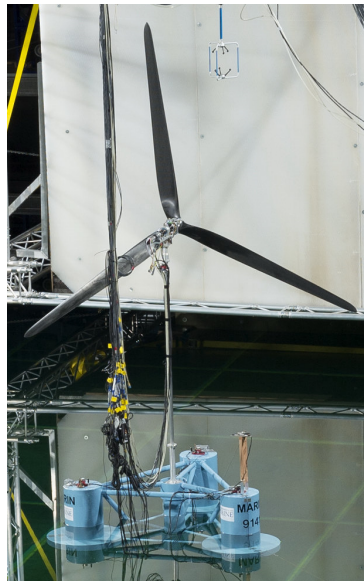
Fig. 3.11: OC4-DeepCwind Semi-Sub system as tested in the ocean basin at MARIN. Photo credit: Andy Goupee, University of Maine [E]
