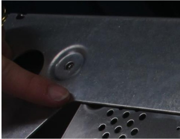
Picture 11-8: Screw covered by metal plate, making disassembly difficult.
