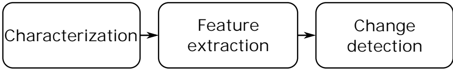
Figure 1: Flow chart of most available model based methods for fuel cell fault detection.
